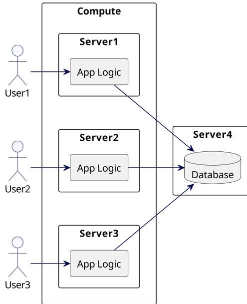
**Figure 1.4** *Scaling compute with multiple servers*
