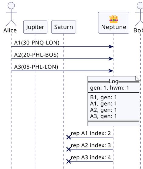
**Figure 2.23** Nodes missing replication of log entries
