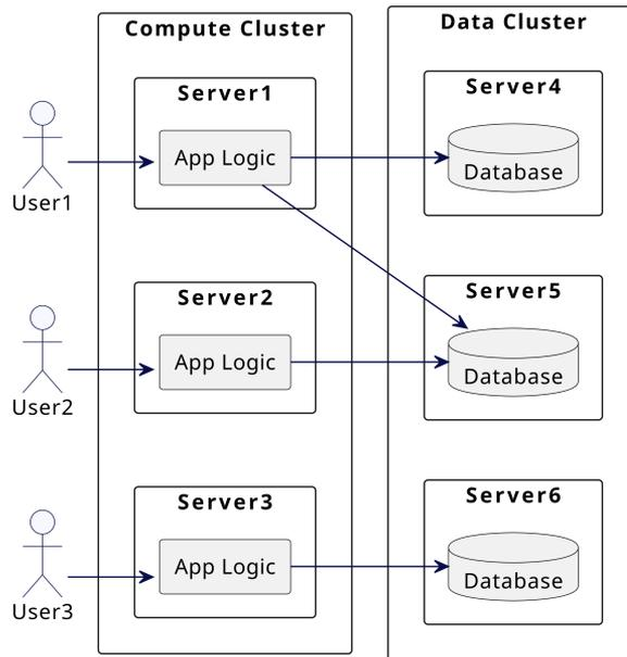
Figure 1.5 Scaling data by distributing on multiple servers
