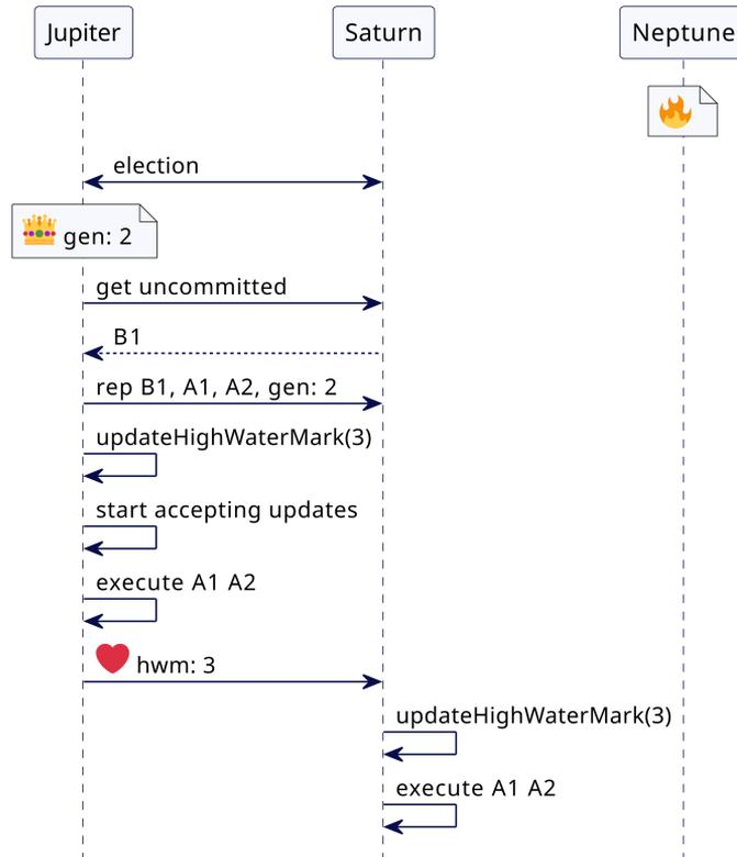
Figure 2.25 New leader replicates missing log entries and High-Water Mark.
