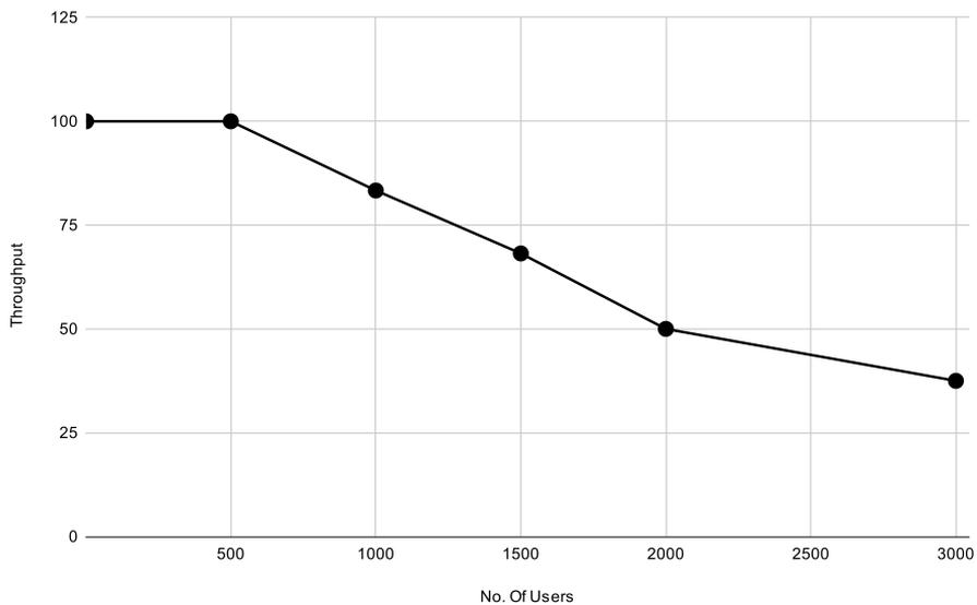
**Figure 1.2** *Drop in throughput with increase in requests*
